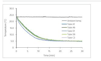
The graph above shows how sample temperature is maintained in the ID7000 AutoSampler when using a 24-position tube rack. Temperature measurement for tubes at multiple positions indicate that they maintain cooling over time when used in a 23°C ambient environment.
