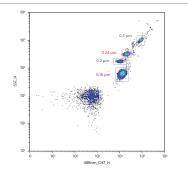
The ID7000 can detect small particles. The figure shows how a mix of fluorescent beads of varied diameters available as a commercial product (Megamix, Biocytex), is analyzed to clearly resolve the 160-nm beads from all other beads and separate from noise, using SSC and channel 7 of the 32-channel PMT array on the blue laser deck.
