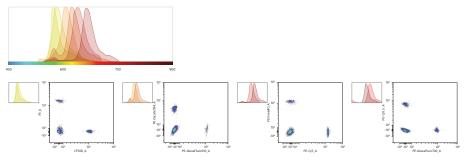
C. Multiple fluorochromes with overlapping emission profiles excited by the 637-nm laser
