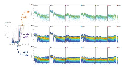
An unstained lysed whole blood sample was analyzed with the ID7000 cell analyzer to understand the contribution of cellular autofluorescence. **A.** The figure shows spectral ribbon displays when studying the gated populations of lymphocytes, granulocytes, and eosinophils. Removing the signal due to this autofluorescence by using spectral fingerprints obtained in the analysis, increases the precision and quality of results.
