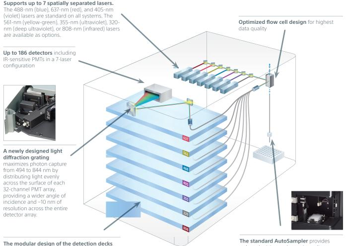
allows each deck to be installed independently, providing the flexibility to perform field upgrades. The standard AutoSampler provides onboard mixing and sample cooling capabilities to simplify operation and ensure accurate results.
