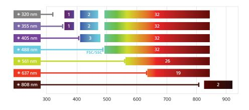
The detection capacity of the ID7000 spectral cell analyzer spans from 360 nm to 920 nm in the 7-laser configuration. The signal is captured using a combination of 32-channel PMT arrays and individual PMTs. The signal above 800 nm is detected with specialized InGaAs PMTs to ensure data quality.
