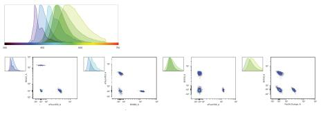
B. Multiple fluorochromes with overlapping emission profiles excited by the 561-nm laser
